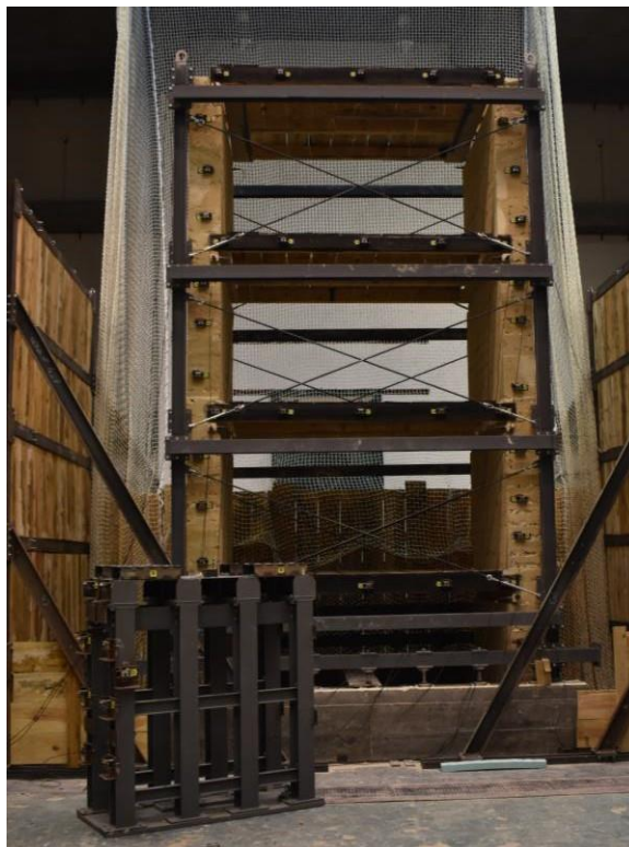
Figure 1 - Metallic shelter and building structure before the trial.
