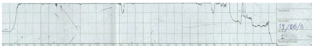
Figure 2 – Obtained graphic of the R1 beam of the pavement, through resistograph.
